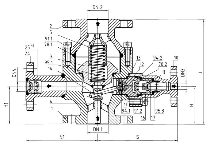
$Figure \ 5\ SSV\ 18/20\ with\ integrated\ non-return\ valve\ and\ multistage\ pressure\ and\ flow\ reduction\ in\ the\ bypass$
